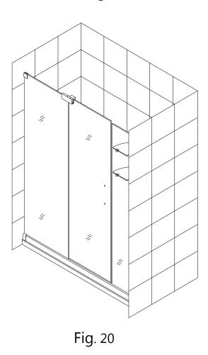
18. Press the **Magnetic strip (19)** on the vertical edge of the **Glass door** and the **Stationary glass 2**.
