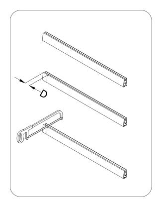
3. Fasten the Guide rail connector (11) to one of the sides of the Guide rail (05). Slide in two Roller assemblies (13) from the other end of the guide rail. Fasten another Guide rail connector (11) to the other side of the Guide rail. Place the Guide rail in the designated position on the base or the threshold and mark the holes through the predrilled holes on the flange of the Guide rail connector.
