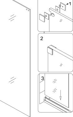
Outline the position of the Wall bracket (17) on the wall. Set the door aside. Remove the Wall bracket from the Stationary glass and by replacing it to the outlined position mark the hole on the wall.
